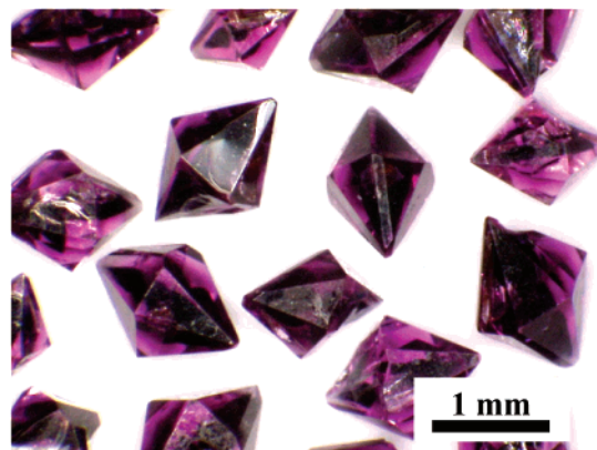
Figure 1. Optical micrograph showing ruby crystals grown from \text{MoO}_3 flux.
